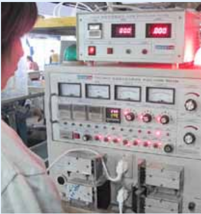
The testing machine alarm is triggered and blinks red if something is wrong with the multi-way socket.
