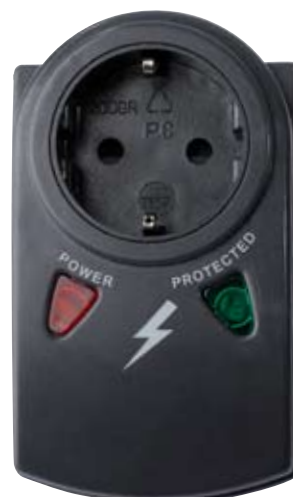
Surge protector. Extra-powerful surge protector with nine protective components. Five variable resistors, including two extra-powerful, three fuses and one gas discharge tube. Signal light that indicates full protection. 230V/16A. Grounded with childproof socket. 36-3390
